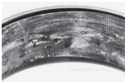
Adhesion on ball bearing
