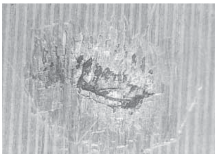
Surface fatigue on ball bearing
