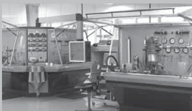
Just one example of the numerous filter testing procedures: Multipass test rig.
