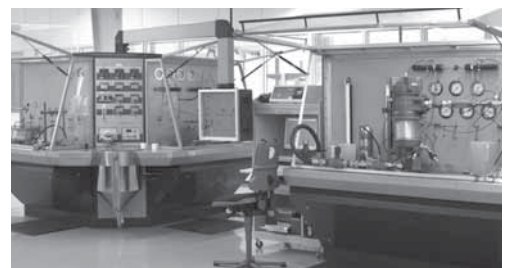
Just one example of the numerous filter testing procedures: Multipass test rig.
